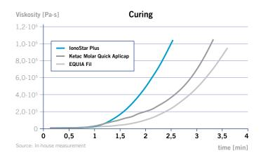
The diagram shows the curing behaviour of the tested materials, measured by rheometer at 37 °C mouth temperature. Thanks to its initial, low-viscosity, consistency lonoStar adheres perfectly to the cavity walls. It then sets rapidly, resulting in only a short wait before the finishing process can begin.
